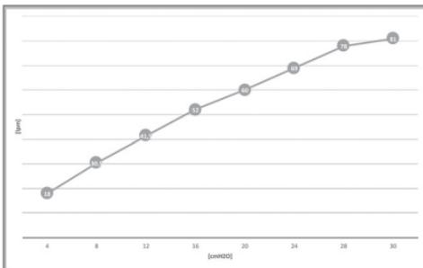
\*Due to machining differences, the outflow from the exhalation orifices may vary ( $\pm 10\%$ ).
